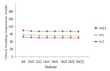
Fig.3 Mesh Convergences for PFGM with various mesh counts
