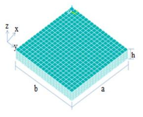
Fig.2 Geometry and dimension of FG Flat Plate
