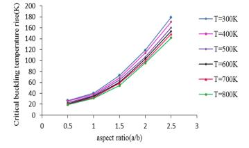
Fig.7 Variation of critical buckling temperature rise with the aspect ratios for Clamped FG flat plate (n=2&a/h=100)
