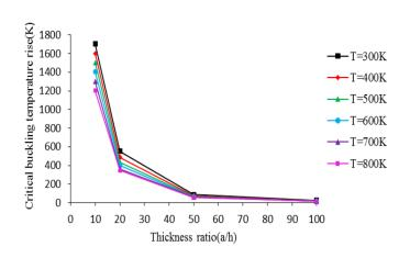
Fig.5 Variation of critical buckling temperature rise with the thickness ratios for Clamped FG flat plate(a/b=1&n=2)
